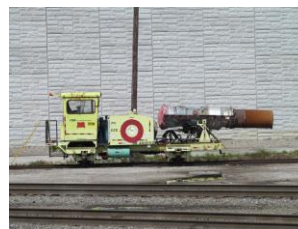
Left: CSX jet propelled MOW equipment at Osborne Yard. Actually it is a jet snow blower. Photo by Bob Dawson
