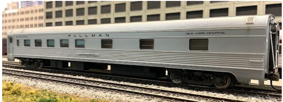
Right: Russ Weis’ HO “Onondaga Valley Pullman.” Russ replaced the trucks and added body mounted couplers along with other modifications to this AHM/Rivarossi Pullman.
